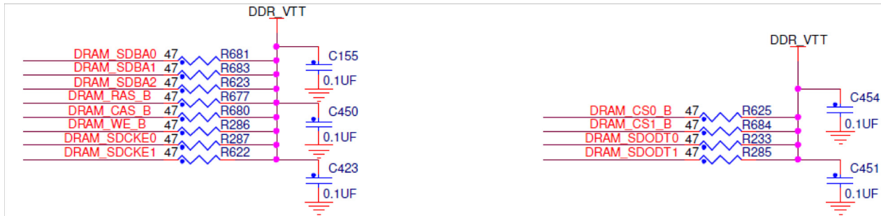
Figure 3-30. DDR_VTT evaluation board examples
